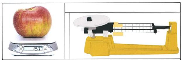
Both of these instruments are balance scales. Even though both balances measure mass, they show mass in different ways. The scale on the left is digital. The scale on the right is a triple beam balance that you operate by hand.
